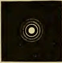
Fig. 68.—Appearance of diffraction rings round a star when the object-glass is properly adjusted.
